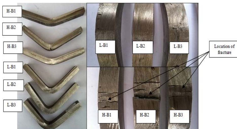
Figure 8. Bend tested specimens showing the location of fracture on low and high heat input welded joints
